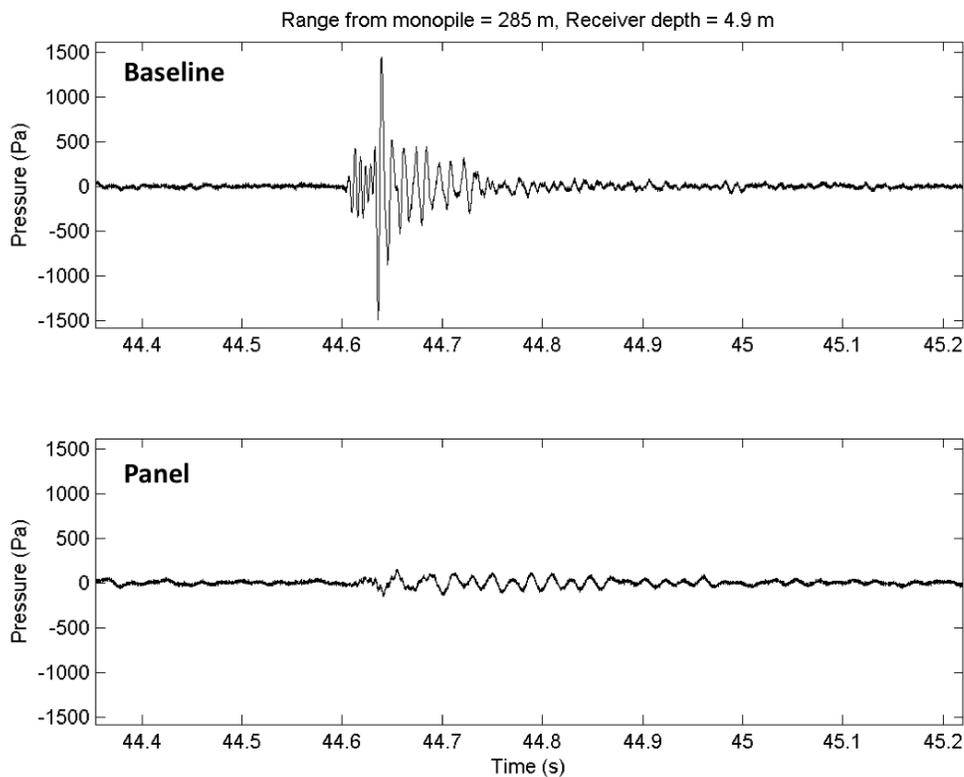
**Fig. 4: Example raw acoustic data from a single event from monopile BU-21 recorded at a distance of 285 m from the monopile. The data from each hydrophone were recorded simultaneously. The acoustic signals correspond to the same hammer strike. The reduction in amplitude recorded by the panel embedded array is due to sound absorption by the acoustic resonators inside the panel.**
