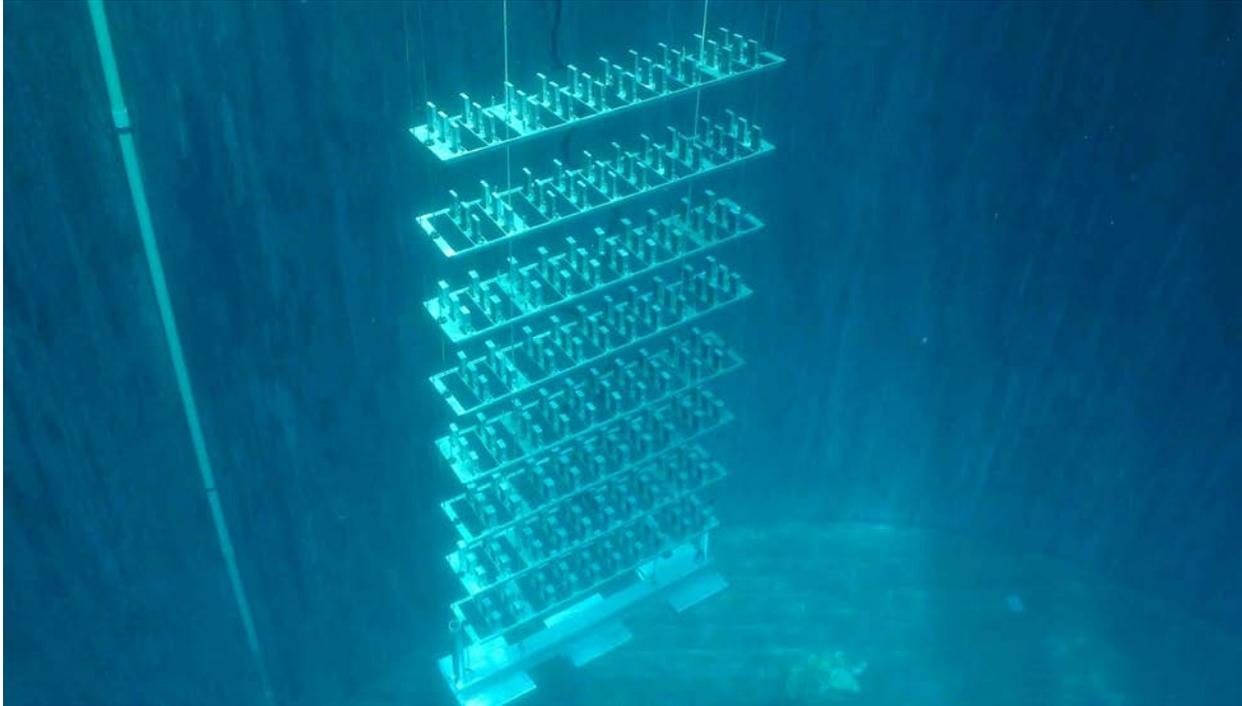
**Fig. 2: Photograph of the fully extended demonstration panel in the ARL:UT test tank. Underwater photographs were made during the Butendiek demonstration; however, the test tank photo more clearly shows the system due to water clarity.**
