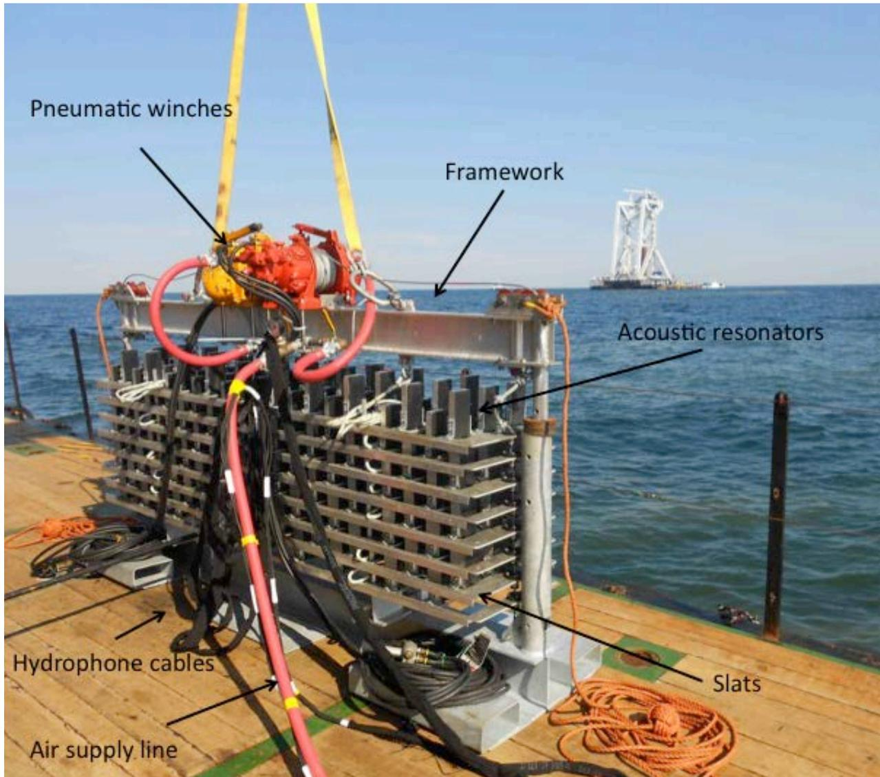
**Fig. 1: Photograph of demonstration panel in collapsed state on deck of the Mena C. The various components of the system are labeled. Note that for the production version of this system, the hydrophone cables, winch control lines, and tag lines will not be present.**
