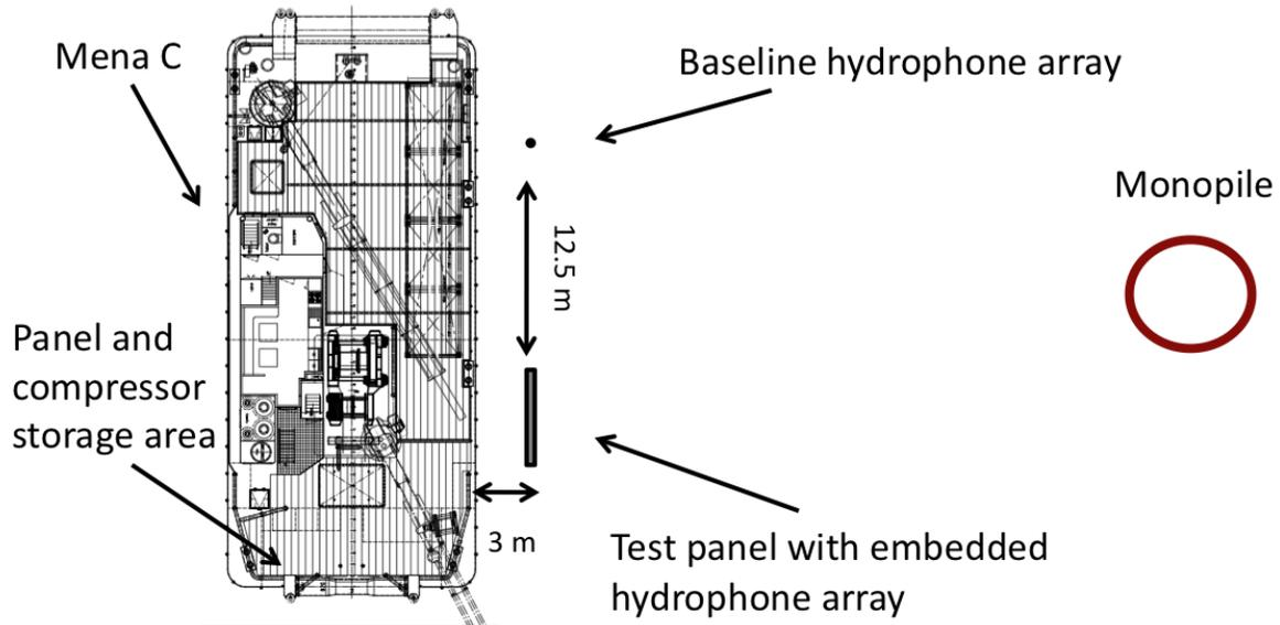
**Fig. 3: Diagram depicting the deployment and test configuration for monopiles BU-32 and BU-21.**
