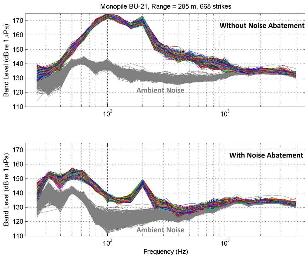
**Fig. 6: One-third-octave band levels for all monopile strikes recorded at the location 285 m away from monopile BU-21. The colored lines are the band levels corresponding to each pile strike. The grey lines are non-pile ambient noise band levels from the quiet sections of data between pile strikes. The horizontal axis is frequency, given in a logarithmic scale.**
