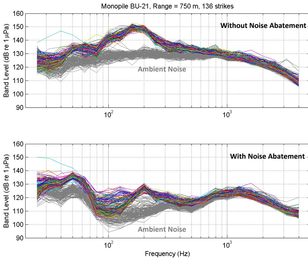
**Fig. 7: One-third-octave band levels for all monopile strikes recorded at the location 750 m away from monopile BU-21. Radiated noise from the monopile was reduced to the local ambient noise levels by the demonstration panel.**
