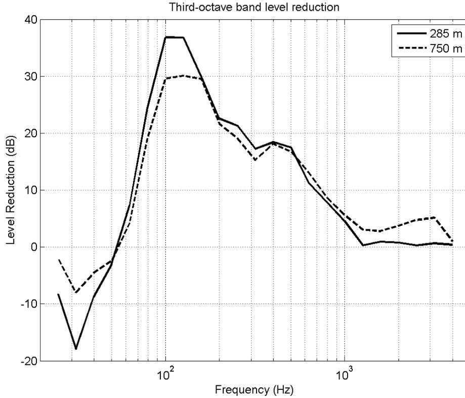
**Fig. 8: Average one-third-octave band level reduction measured at each of the test locations for monopile BU-21. The slightly reduced noise abatement levels at 750 m were due to the fact that the noise was fully reduced to the ambient noise level.**
