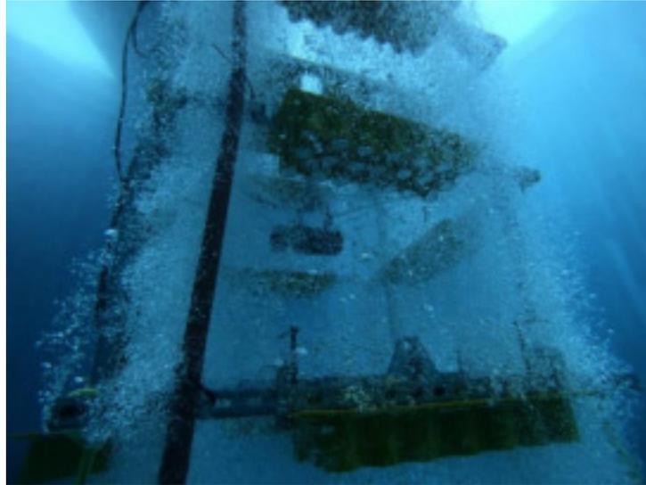
***Photograph of the resonators being filled with air during testing. The results showed the resonators can be filled with compressed air and that the compressed air increases the performance of the system***
